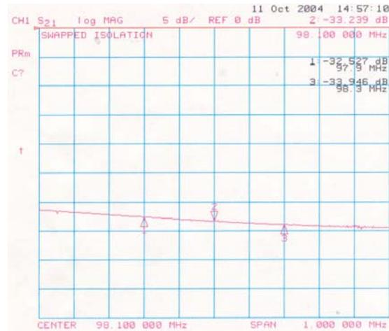
Although these antenna tests demonstrate very high isolation, just a bit more might be desirable for some installations. The FM-7380 circulator-isolator is suggested, where required, to provide up to 32 dB additional isolation. Some installations have found the isolator is not needed. Jampro suggests budgeting for this inexpensive accessory and install it if needed or if recommended by the HD transmitter manufacturer.
