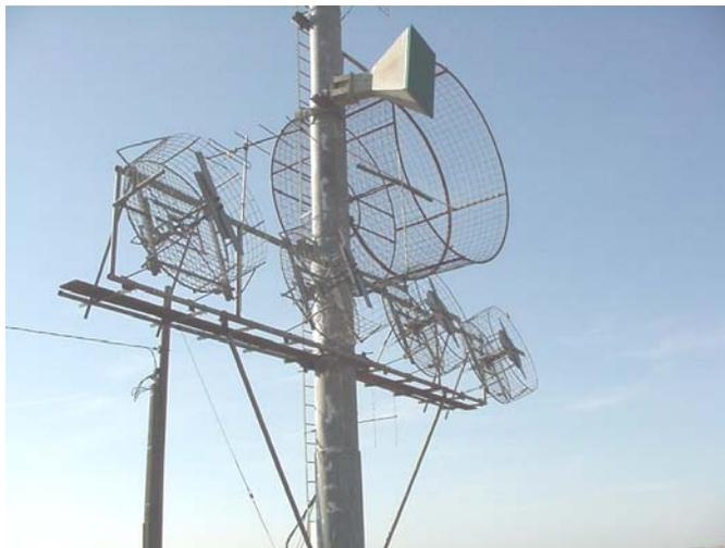
The RF point source is located multiple wave lengths ( ~ a mile) away from the antenna turntables to provide the signal used by your antenna while under test. The sources are operated from the control center at the base of the turntables. Several antennas can be under test at any give time. The source RF generators work for FM and TV antenna systems.
