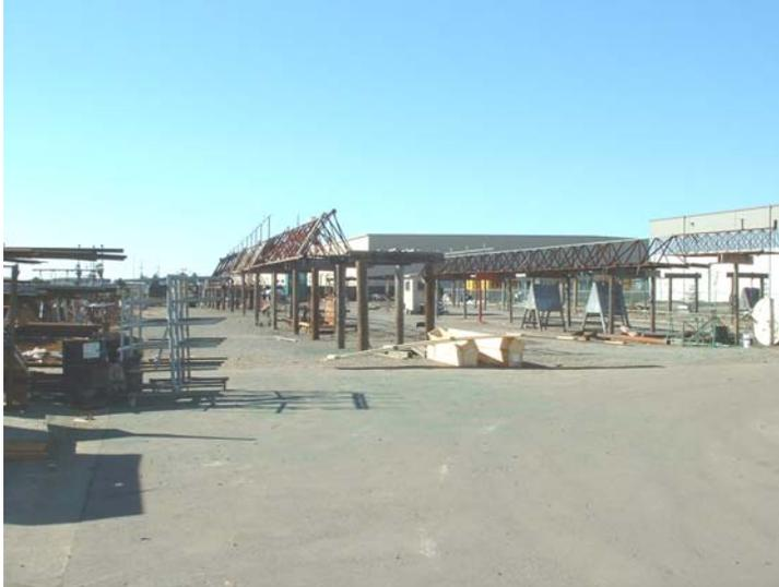
The 'back yard' where a large quantity of sample towers are stored for full size testing. Full size VSWR setting is also done here. This assures meeting the VSWR antenna specification with virtually no field 'tweaking' when the antenna is mounted on your tower.
