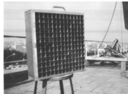
Fig. 10 – Reflectarray used in the 60's to validate finite array modelling [17]
