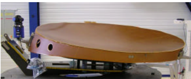
Fig. 9 - Polarisation sensitive shaped reflector: thin gridded Kevlar front skin + CFRP rear dish + intermediate stiffening structure (courtesy Astrium I)
