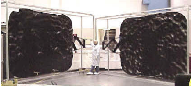
Fig. 7 – Shaped reflectors for INTELSAT contoured beam coverage (Courtesy H. Wolf Astrium-D)
