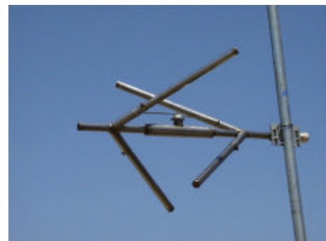
Fig.2 – JAMPRO's Circularly polarised FM broadcast antenna “Penetrator” [3][4]
