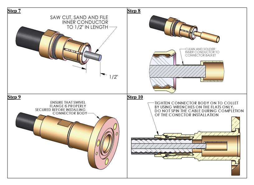
Pressure test cable and connectors to ensure proper installation of connections. Congratulations, you have completed installation of the 7/8" EIA foam cable connector.
