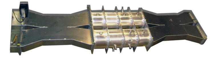
Waveguide constant impedance cross-coupled combiner provides the high isolation needed for adjacent channel combining applications. The RWCE series combiners consist of two RWBE filters placed between two RWHE 3-dB hybrids. Out of band reflections are absorbed in the supplied absorber load. This system allows different high power UHF channels to combine & use one common antenna /feed system while still maintaining low insertion loss.
